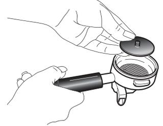
Insert the rubber disk into the filter holder.
