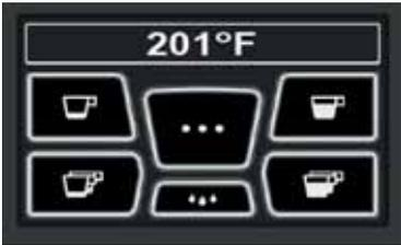
Push the button to be programmed (e.g. key 1): the icon of the key in question remains selected on the display. When the desired level is reached in the cup or cups, press the key again. Continue with any additional programming of the coffee buttons.
