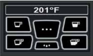
Place the cup or cups underneath the filter holder nozzles. The numbers relative to each key appear on the group display.
