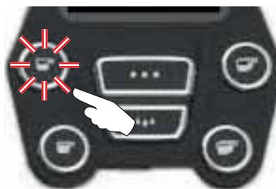
During this phase, the value of the pulses of the volumetric dispensing device (at the top right-hand side of the display <sup>(\*)</sup>) increases. When the button is released, the value reached is recorded and appears under the key programmed.
