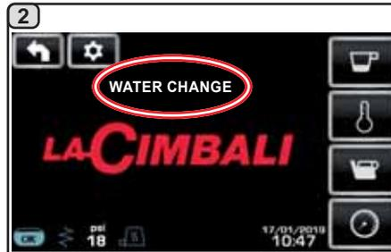
2 The following message will be displayed: "WATER CHANGE". The water from the boiler will drain from the hot-water nozzle (60 - 70% ca. of the total capacity).
