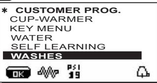
Use the ▲ and ▼ keys to position the cursor (black line) on the desired line and then press the ► key.
