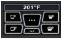
By pressing one of the coffee keys (e.g. key 1), the relative water dose is shown on the services display and the icon of the key in question remains highlighted on the group display.
