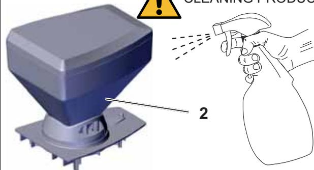
6 Wipe the inside with a damp, absorbent cloth to remove all dirt and dry if necessary. Make that the hopper (2) is completely dry before refitting it onto the grinder-doser.
